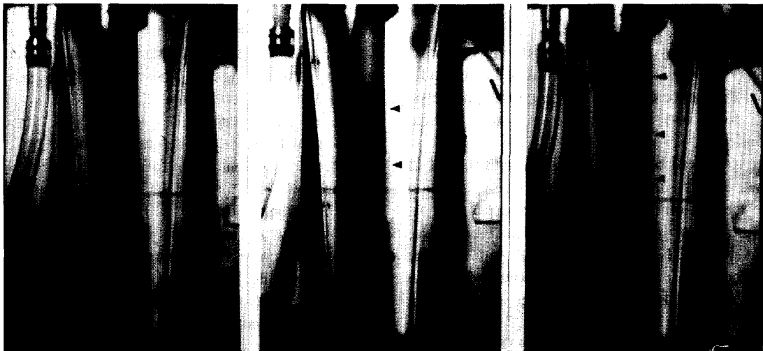
Fig. 4. Focusing of hemoglobin. The gray cylinder in the center of each picture is the packed bed. (left) The bed is completely filled with 0.1% (w/v) hemoglobin solution, t=0 . (middle) Progression to a focused band at 3 h; the arrowheads mark the edges of the partially focused band(s). (right) The major band is focused between the arrowheads just above the center mark. There is also a secondary band near the top arrowhead, focused on the right-hand side of the bed.
